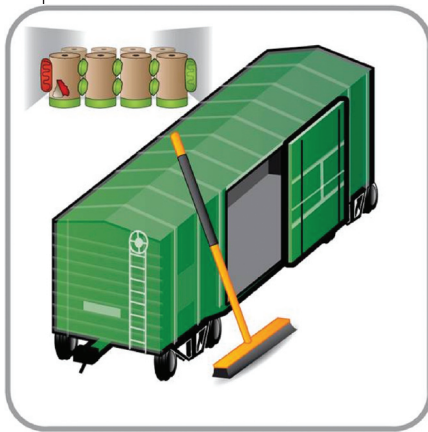
Figure 1: Each car loaded has its own picture with colors indicating received in good condition (green) or damaged (red). The visualization of the car also indicates that it was received in good working order and clean.
